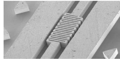
Fig. 4. Structure of Interdigitated CPW
