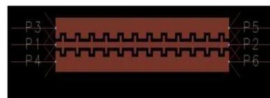
Fig. 5. Layout of Interdigitated CPW
