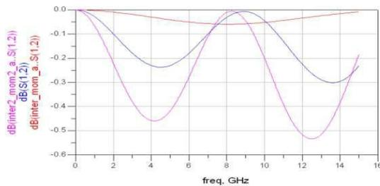
Fig.13. Interdigitated CPW of various thickness for filter 2(insertion loss)
