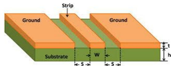
Fig. 1. Structure of the CPW
