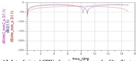
Fig.12. Interdigitated CPW of various thickness for filter 2(return loss)
