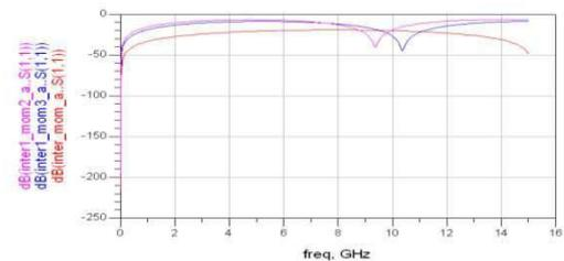
Fig.10. Interdigitated CPW of various thickness for filter 1(return loss)
